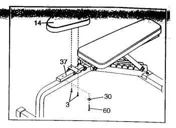
24. Make sure that all parts are properly tightened before you use the weight bench. The use of all remaining parts will be explained in ADJUSTING THE WEIGHT BENCH starting on the following page.
